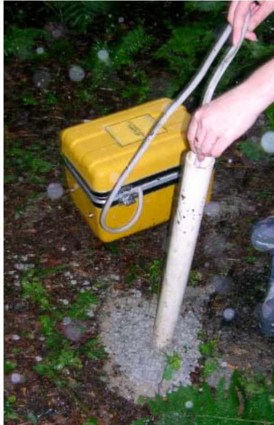
Figure C4: To develop the well, pump it until the water coming out of the pump is clear. For this process, a peristaltic pump was used.
