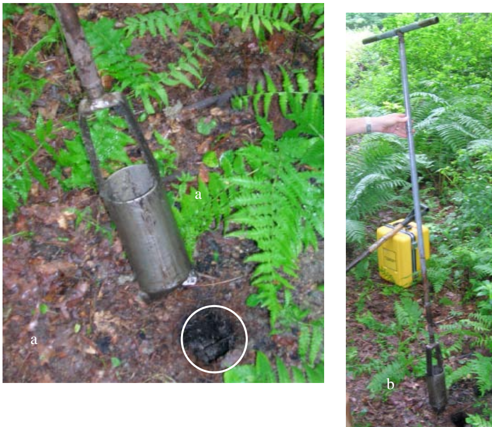
Figure C2: (a) A close up view of the bucket auger with the bore hole (circled in white). (b) The bucket auger.
