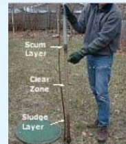
Measure scum & sludge layers. Pumping needed if combined layers are >50% of tank volume.
