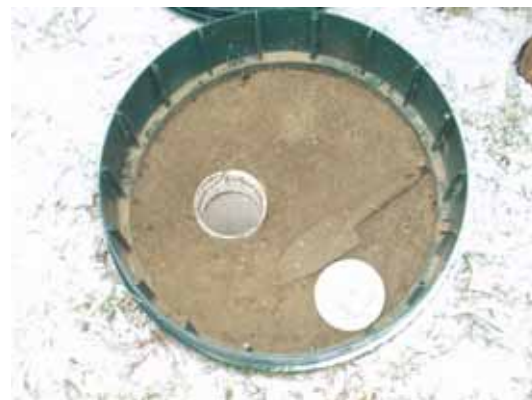
Groundwater sampling port downgradient of wood chip bioreactor at URI Peckham Farm.
