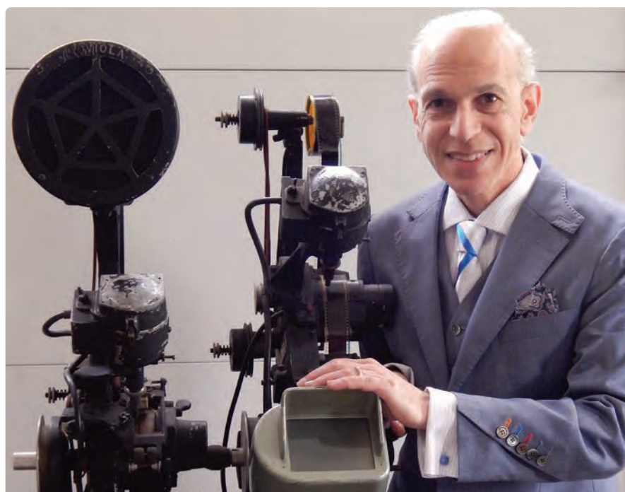
Tom Ohanian, M.B.A. '14, with a Moviola Model DX manufactured in Hollywood, circa 1924. The Moviola, a film viewer, was used in the editing process. At the time, editors had to physically cut the film and splice it to the next appropriate piece.
